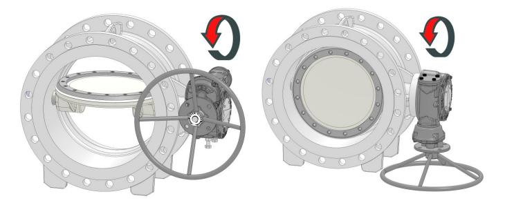
**c.** Place the valve on its flange. The retaining ring must point upwards. For big size valve you may need a support under the valve.
