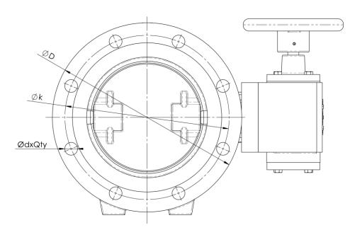
ØD:Outside Flange DiameterØk:Hole Circle DiameterØdxQty.:Diameter of Bolt Holes x Numberof Bolt Holes
