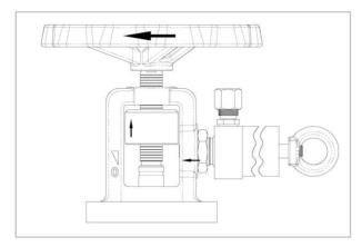
Turn the hand wheel (2) in closing direction (clockwise) until the piston rod (4) in the cylinder comes out and holds the setting nut (3) in its upper position.
