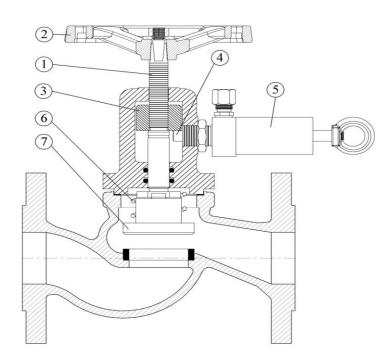
The valve is a stop valve with a remote quick closing function but can also serve as a conventional stop valve by using the hand wheel (2).
