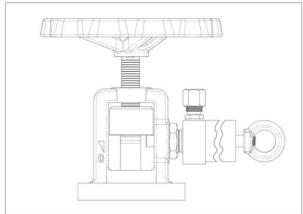
Stop the turning of the hand wheel (2) when the mechanical stop is felt and the setting nut (3) is in hard contact with the thread the end of the stem (1).
