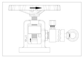
Turn the hand wheel (2) in opening direction (anticlockwise).
